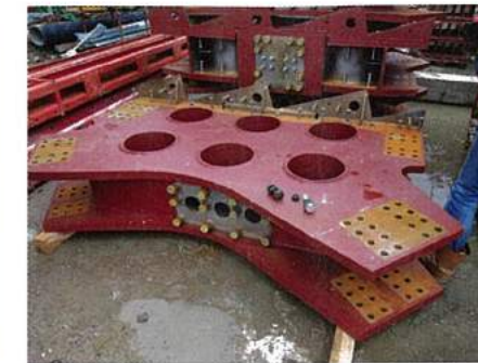
↓ FIGURE 13: Concrete-to-steel connection
